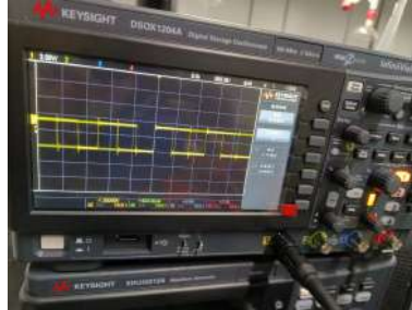
Figure 7.4: PWM signal sent to the WS2812B lights
