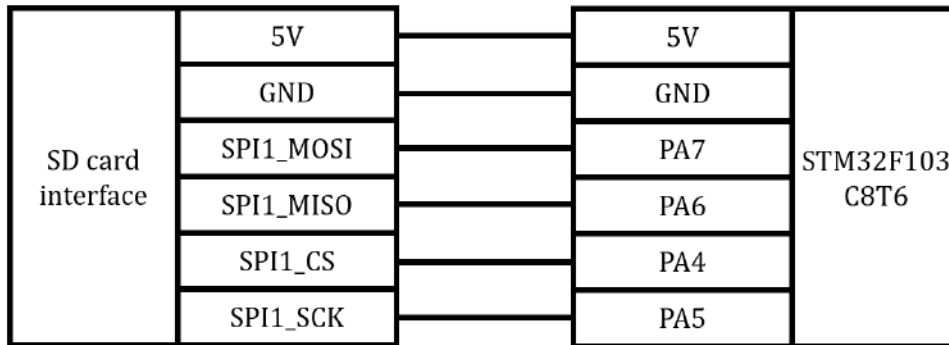
Figure 6.3: Illustration for SD card interface and MCU connecting
